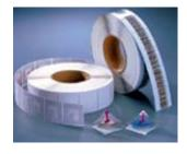
These tags are essentially an LC tank circuit that has a resonance peak at 8.2 MHz. Sensing is achieved by sweeping around the resonant frequency and detecting the dip. Deactivation is achieved by detuning the circuit by partially destroying the capacitor. This is done by submitting the tag to a strong electromagnetic field at the resonant frequency which will induce voltages exceeding the capacitor's breakdown voltage, which is artificially reduced by puncturing the tags
